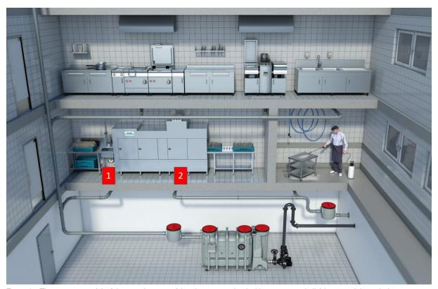
Example: The wastewater (1) of the pre-clearance (cleaning water mixed with greases and oils) is passed through the grease separator. The wastewater from the subsequent mechanical purification stage of the dishwasher (2) then contains only small amounts of grease and might be discharged directly into the sewage system if possible.
